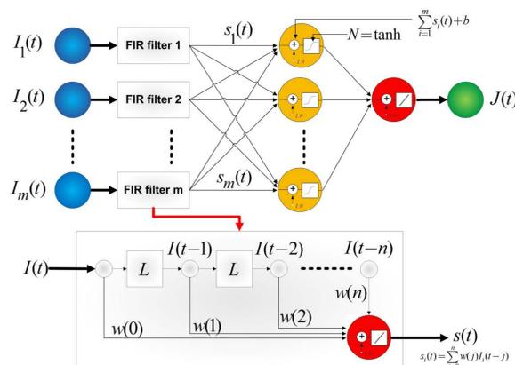
FIG. 2. A schematic diagram of the nonlinear (dynamical) FIR network used in this work.
